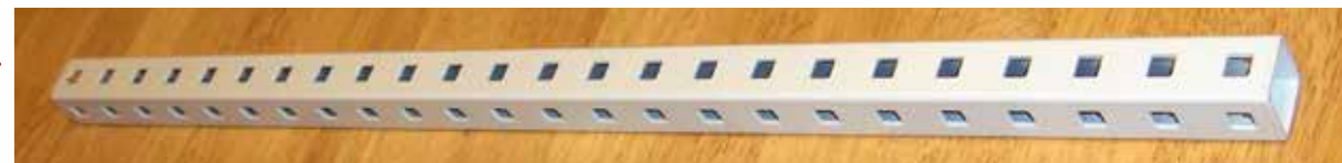
Down Tube (x4) - 1" x 24" square tubing, 5/16" square hole every inch
