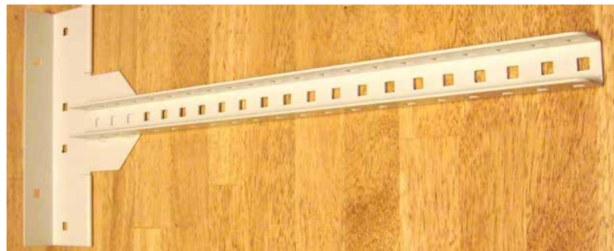
T-Brace (x4) - 1 ¼" channel x 24" w/ 9" angle bracket, 5/16" square hole every inch.
