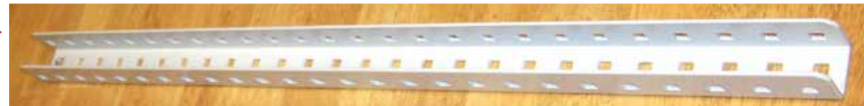
Ceiling Mount (x4) - 1 ¼" x 26" channel, 5/16" square hole every inch
